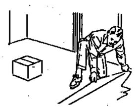
2. As a test, before spreading adhesive, lay pieces of Tajima tile from the center point to one side wall and one end wall.
