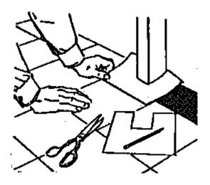
6. To fit border pieces around abstructions, simply make a paper pattern to fit. Trace this onto the tile and cut.
